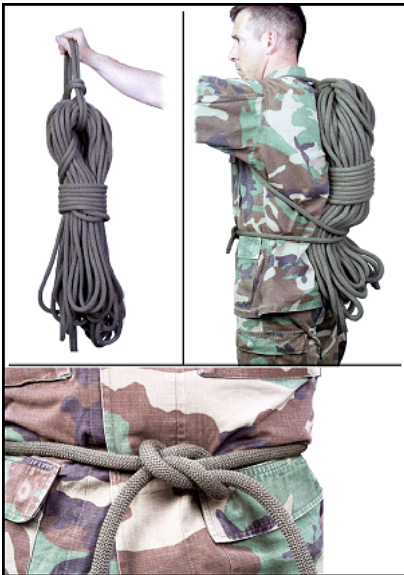
Figure 4-5. Butterfly coil tie-off.
