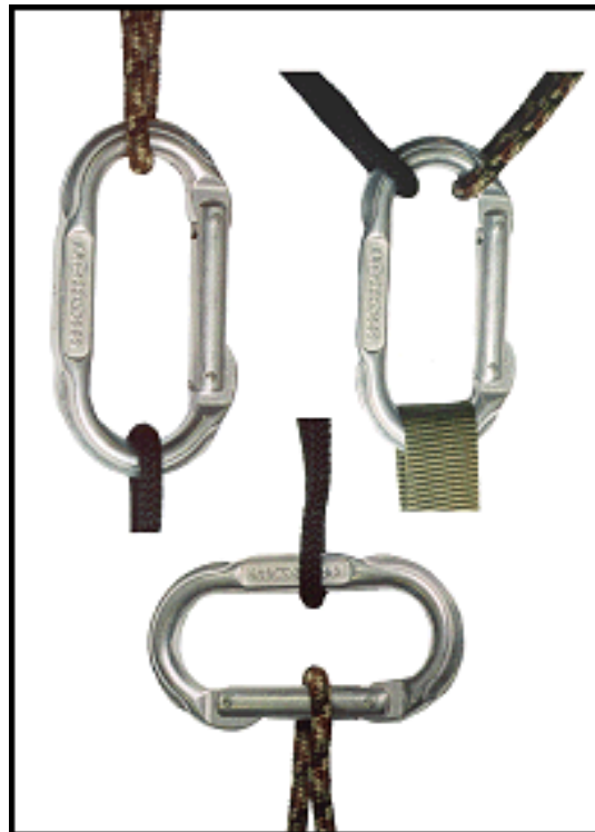
Figure 3-12. Major and minor axes and three-way loading.
