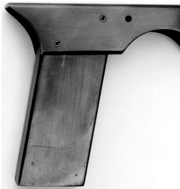
Photo 6: The grip pinned in position
