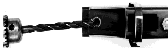
Photo 24: Drilling through the lower receiver bolt holes.
