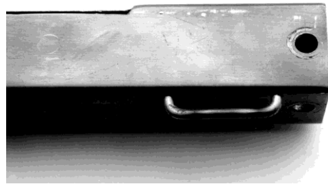
Photo 26: The Sling Loops are silver soldered in place.
