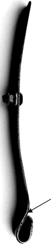
Photo 8: The magazine spring catch
