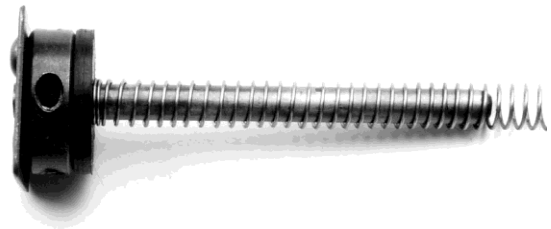
Photo 38: The recoil shield, mainspring and guide rod.
