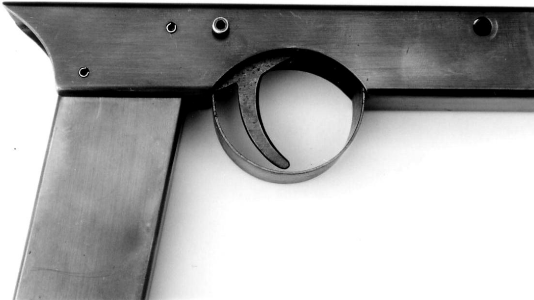
Photo 17: Trigger and guard fitted to receiver
