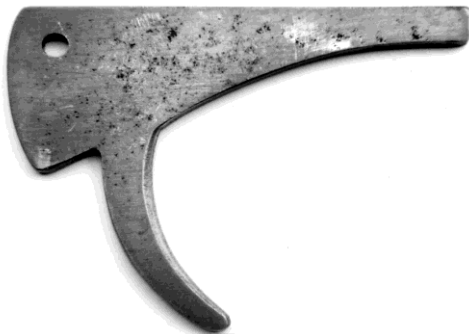
Photo 16: The trigger is cut from a section of steel plate.
