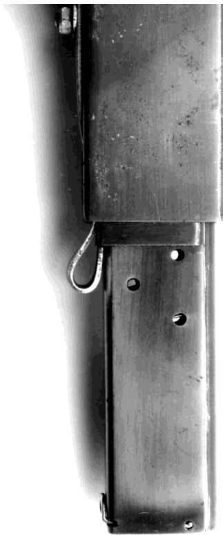
Photo 15: The spring catch holding magazine in place.
