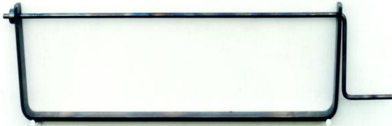
Photo 36: The spring coiling machine.
