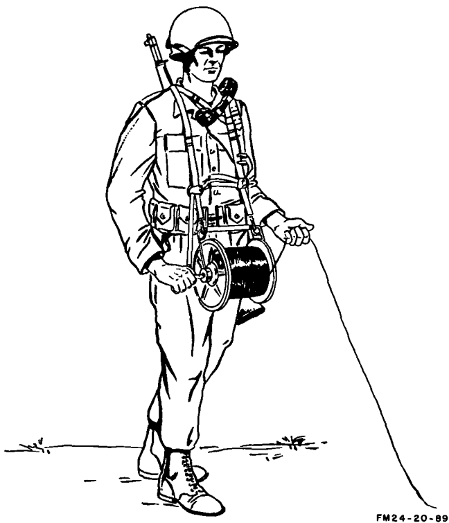
Figure 57. Recovering wire with Reel Equipment CE-11.
